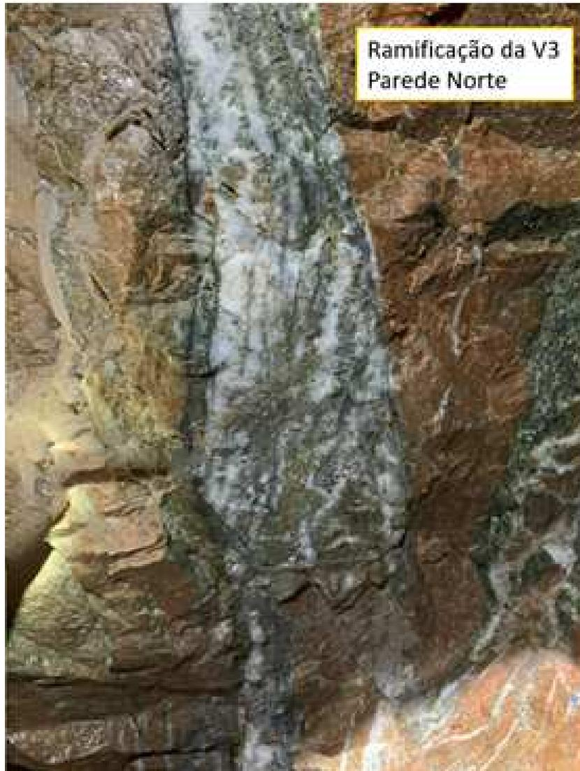
**Figure 2– Intersection of Vein 3 in the Serra ramp showing strong contrast between the mineralized quartz sulphide vein and the pink granite country rock suggesting the deposit should be amenable to ore sorting.**
