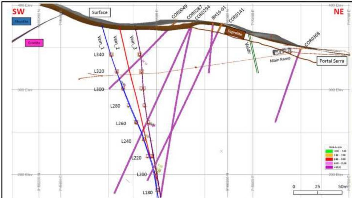
**Figure 4 - Cross-Section showing Serra ramp, three Serra veins and historic drill hole traces**
