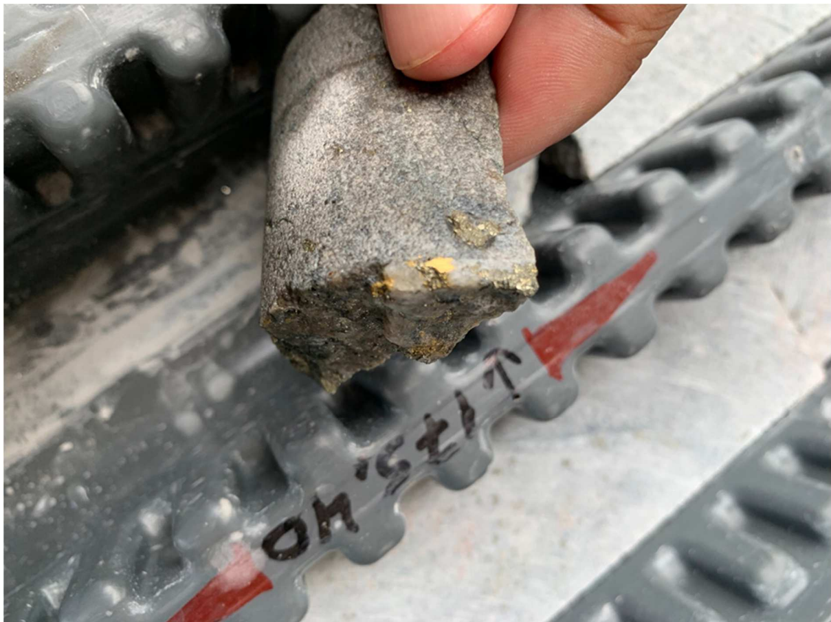
Figure 1 - Visible Gold from 21-SD-010 @ 175.40m down hole depth.
