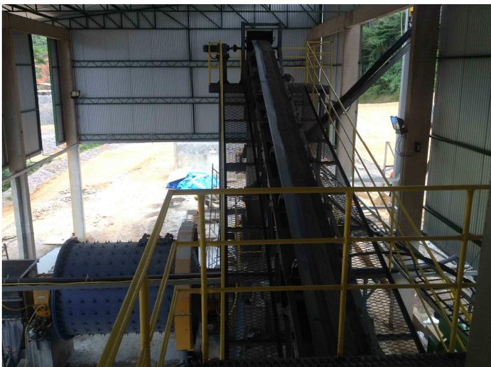
**Ore being fed to Ball Mill**
